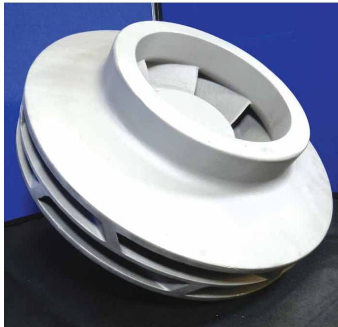
Figure 3: Casting from QuickCast Pattern
